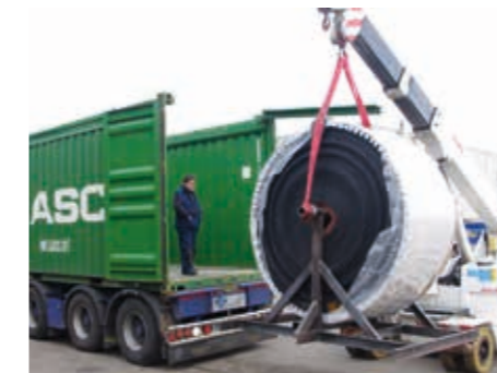
Loading a 8.2 tons Polysur® Ferro elevator belt with crane in a 20' ft. open top high cube container
