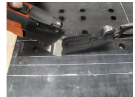
Electric groove cutting tool for fitting the single, double or triple steel vice-part
