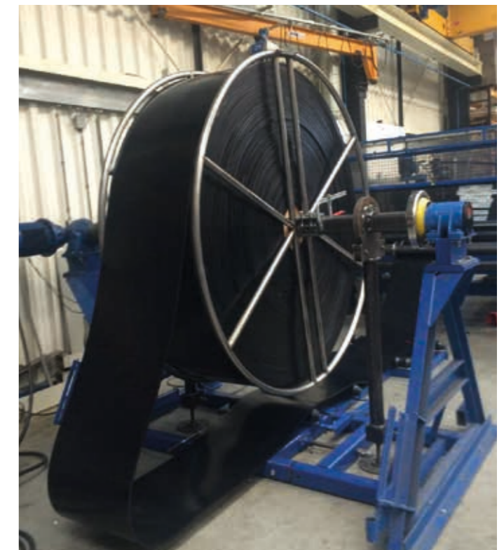
Decoiling the Polysur® Ferro belt in the CNC bolt hole drilling machine
