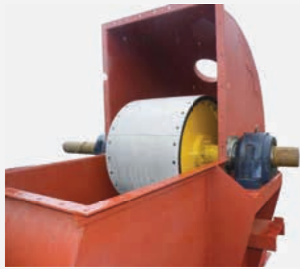
Elevator head section with drive pulley with 'Metallag' sintered all metal pulley lagging
