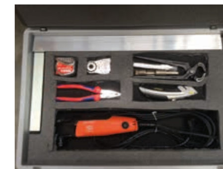
Complete toolbox for preparing other belt end on site to fit the Polysur® Solid belt fastener
