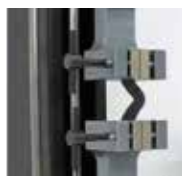
Angle tear strength
