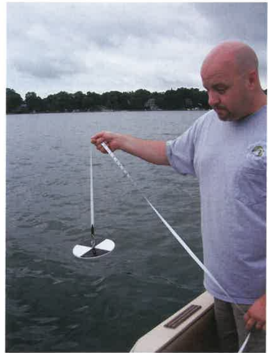
Greg Denny monitoring water clarity with a secchi disk in 2007. Photo by Tori Trauscht.
