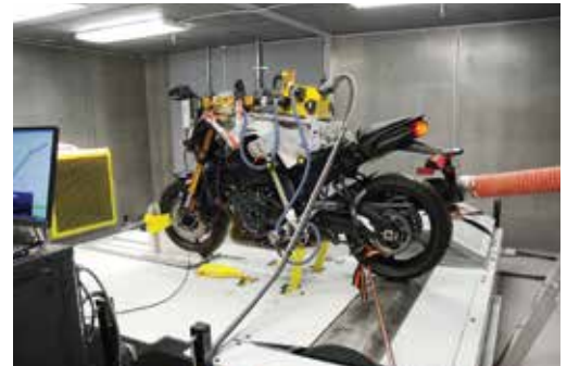
Self-Contained End-Of-Line Test Cells
