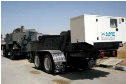
High-Load, Low-Speed Tow Dynamometer
