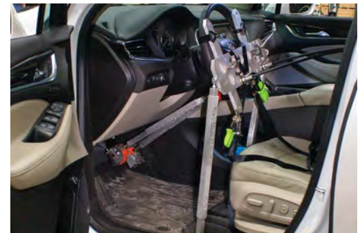
Robotic pedal-throttle actuators for automatic driving
