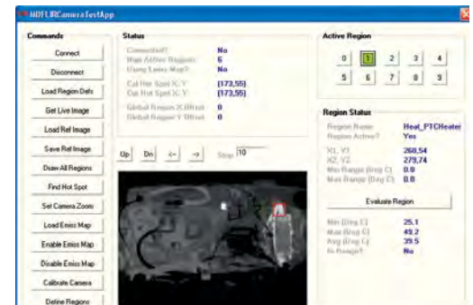
Thermal Imaging and vibration analysis are commonly integrated into EOL test stands. Thermal images on key under hood points before and after cycle testing allows QA engineers to establish pass/fail criteria based on areas-of-interest and temperature limits.
