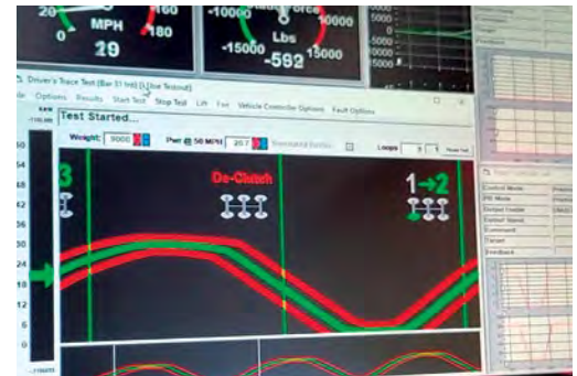
Customizable drive cycles include speeds and grades
