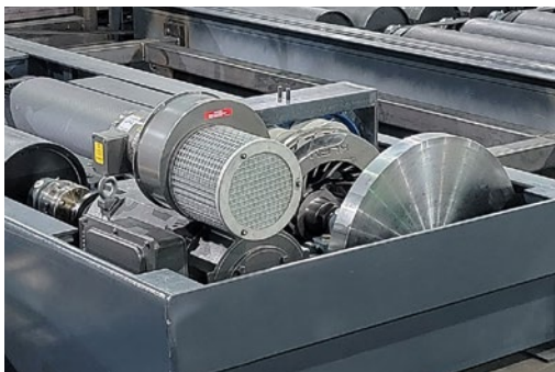
AC Motor, Eddy Current and Inertia Fly-wheel design
