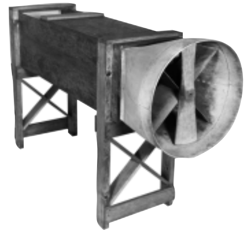
Reproduction of the 1901 Wright wind tunnel, the first wind tunnel to produce reliable aerodynamic data.
