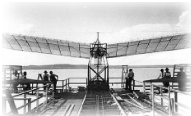
Langley's "Great Aerodrome" perched aboard a houseboat on the Potomac, just before a disastrous launch that tumbled the aircraft down into the river.
