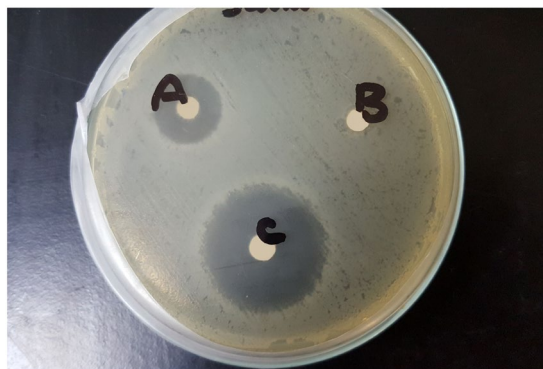
Figure 2. Disc Diffusion antibiotic sensitivity test against Staphylococcus aureus . (a) Pure honey, (b) Chitosan hydrogel, (c) F3 (75% honey + chitosan hydrogel).
