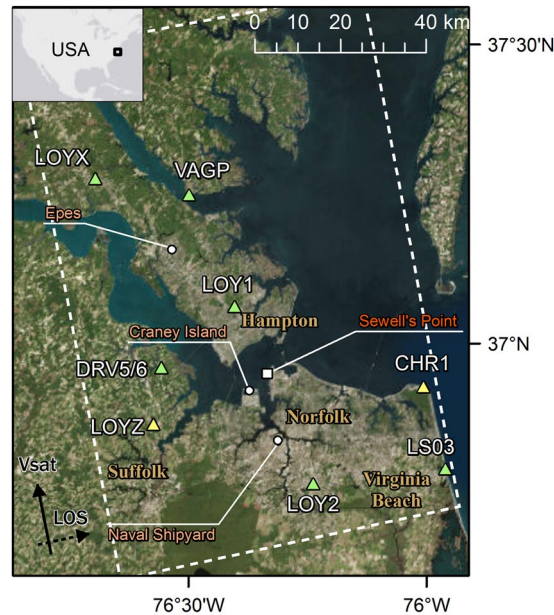
Figure 2. Area of study covering Hampton Roads, showing available GPS stations for reference. Green triangles represent stations used for the GPS reference frame tie-in, while yellow triangles represent stations used only for independent comparison. SRTM topography varies from -55 m to 15 m. The ALOS-1 track used in this study is shown with the dashed line. ArcGIS 10.4 software ( http://www.esri.com/software/arcgis ) was used to generate the figure. Service layer credits ESRI, DigitalGlobe, GeoEye, Earthstar Geographics, CNES/Airbus DS, USDA, USGS, AeroGRID, IGN, and the GIS User community.
