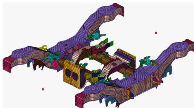
Fig. 5. Finite element model of the bogie frame.
