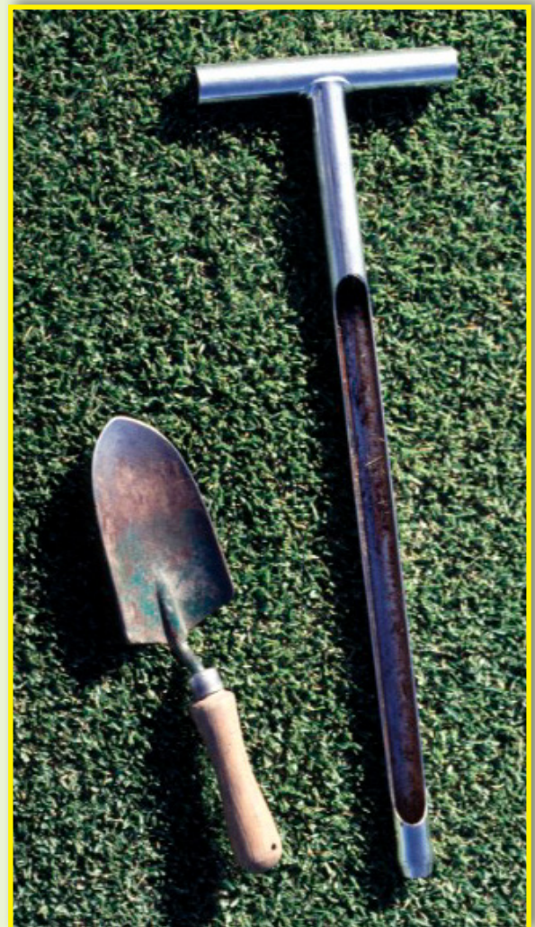
Figure 1. A \frac{3}{4} -inch core sampler and a hand trowel; both are suitable for collecting soil samples. (W. Upham, Kansas State University)
