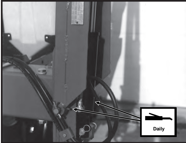
1. Conventional Marker Assembly - 4 Zerks Per Assembly
