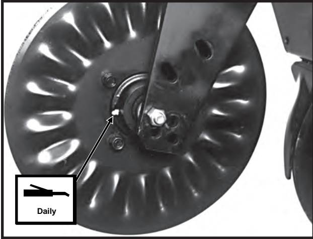
Frame Mounted Coulter Hubs - 1 Zerk Per Hub (Pump grease into hub until grease comes out around the seals. Spin hub while filling with grease.)
