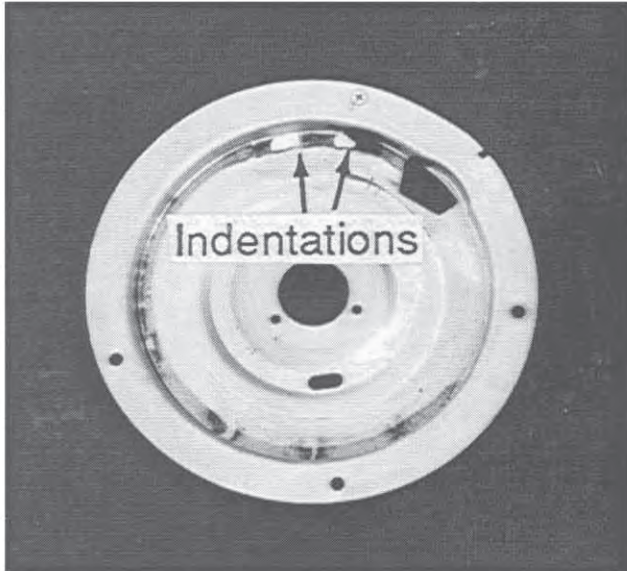
Photo shows worn plate
