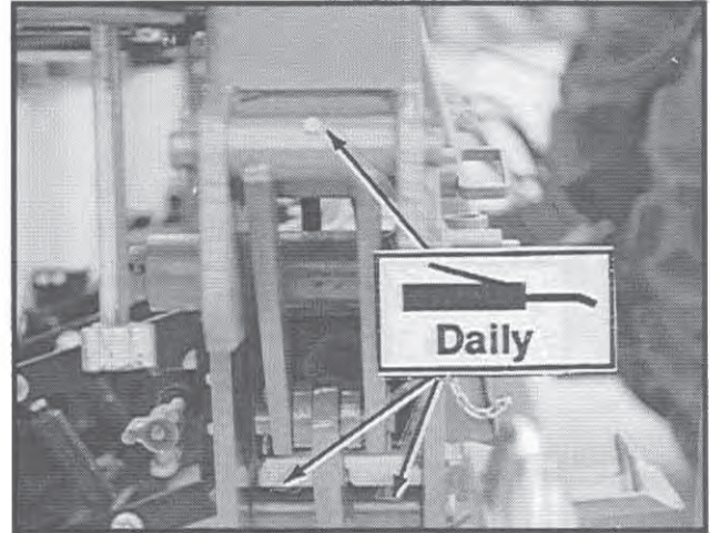
6. Wing Hinge Linkage(Folding Model) - 3 Zerks Per Hinge
