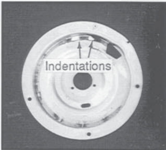
Photo shows worn plate
