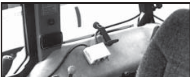
Style B - Point Row Wrap Spring Clutch Control Box
