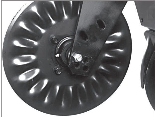
Frame Mounted Coulters Hubs - 1 Zerk Per Hub (Pump grease into hub until grease comes out around the seals. Spin hub while filling with grease.)
