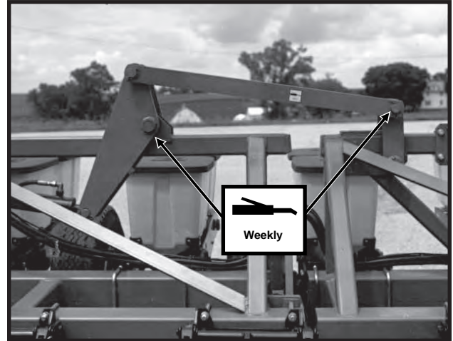
4. Wing Locks - 3 Zerks Per Wing
