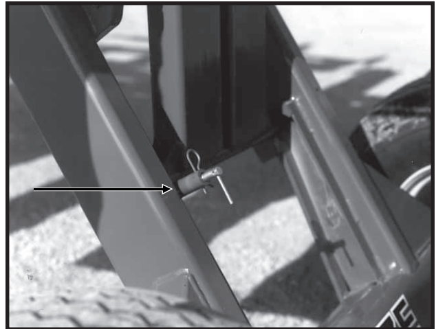
Manual Safety Lockup Pin In Locked Transport Position
