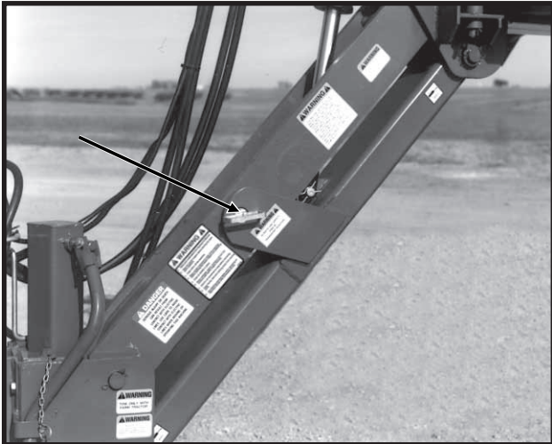
Hitch Parallel Linkage Pin In Transport Position
