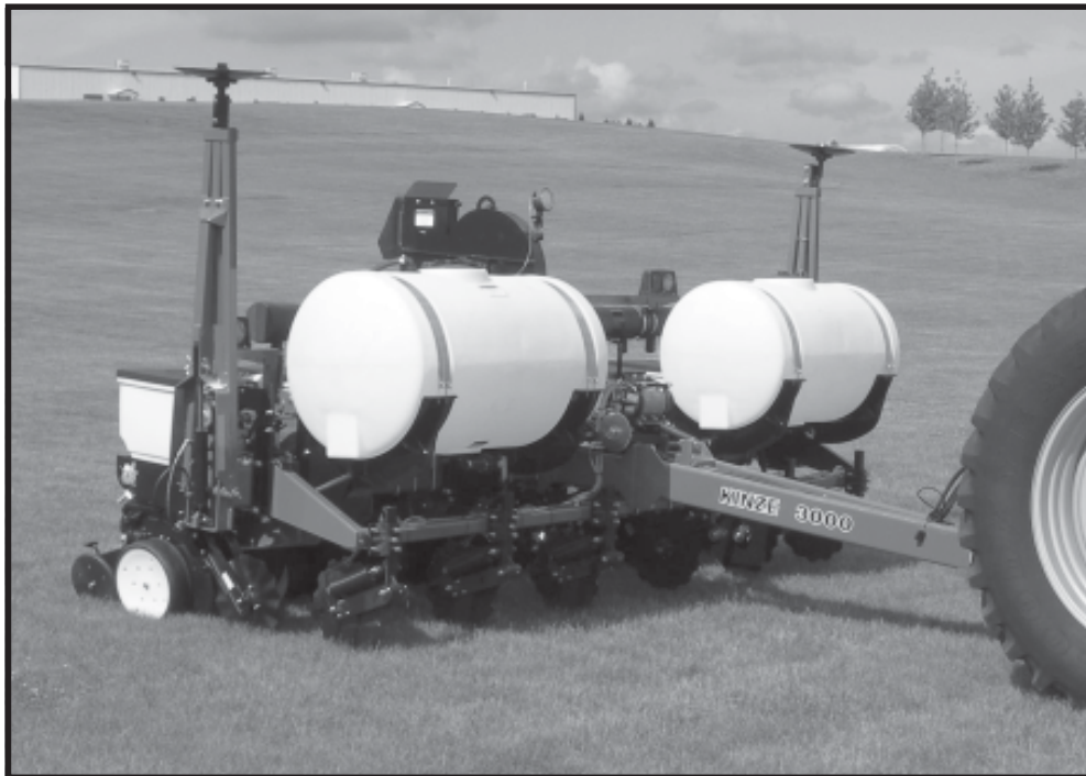
Model 3000 EdgeVac ® 6 Row 30" Pull Type Planter Shown With Liquid Fertilizer, Squeeze Pump And Notched Single Disc Opener Packages Installed
