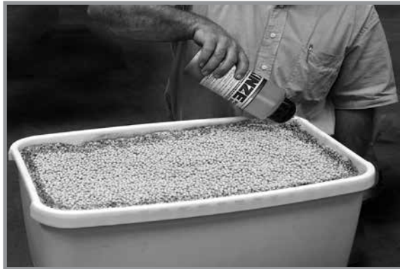
Adding graphite to conventional hopper
