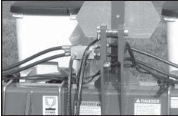
Rigid Frame Machine With Single Valve Hydraulic System
