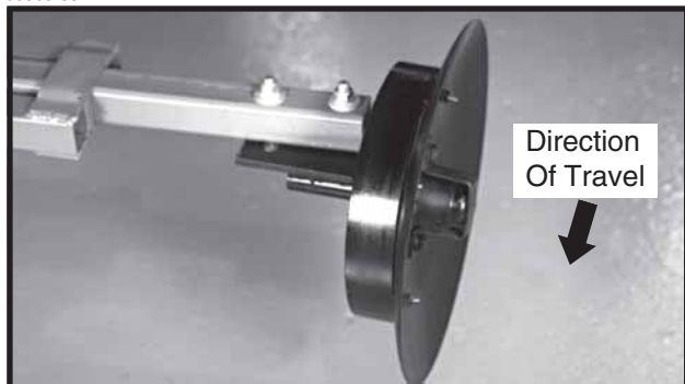
Row Marker Disc Blade Shown With Depth Band (Standard On 8 Row Wide - Up)
