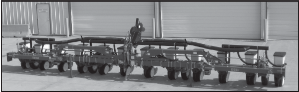
Model 3140 12 Row 38" Planter (Less Optional Row Markers) Shown In Planting Position
