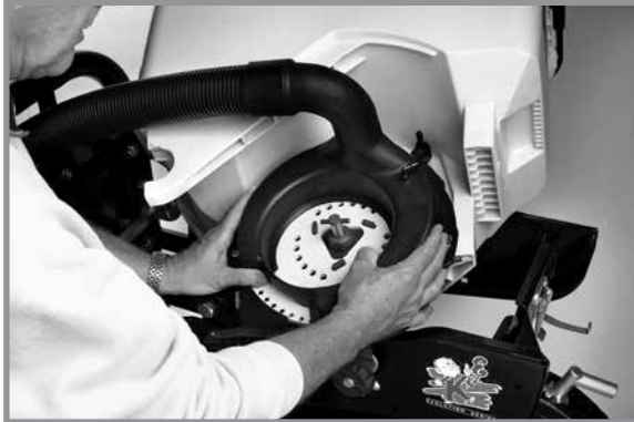
Remove vacuum cover and seed disc
