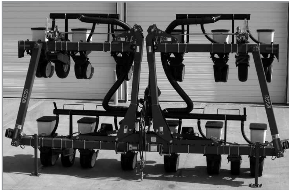
Model 3140 12 Row 38" EdgeVac Planter (Less Optional Row Markers) Shown In Transport Position
