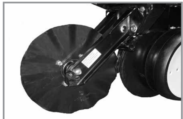
Row unit mounted no till coulters
