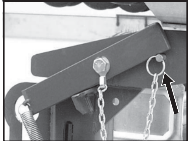
Transport Latch Locking Pin Installed For Transport
