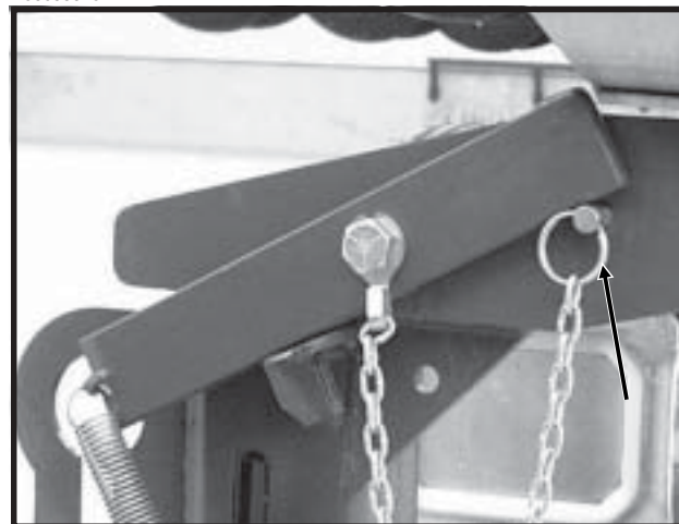
Transport Latch Locking Pin Installed For Transport
