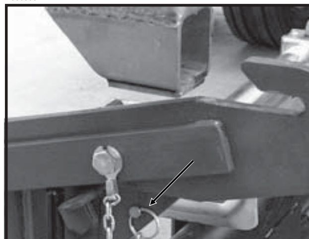
Transport Latch Locking Pin Stored For Field Operation
