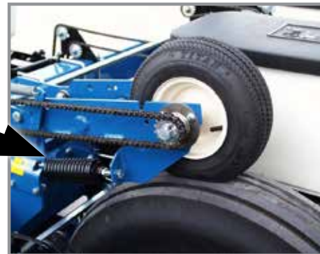
Down pressure spring location
