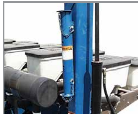
Row marker lockup in storage location
