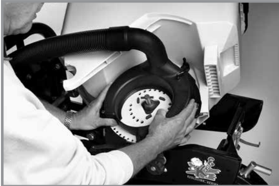
Remove vacuum cover and seed disc
