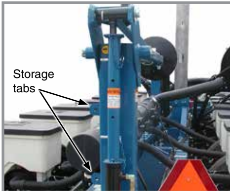
Row marker lockup installed
