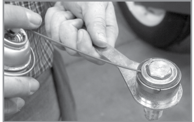
Wrap Spring Wrench Lubrication
