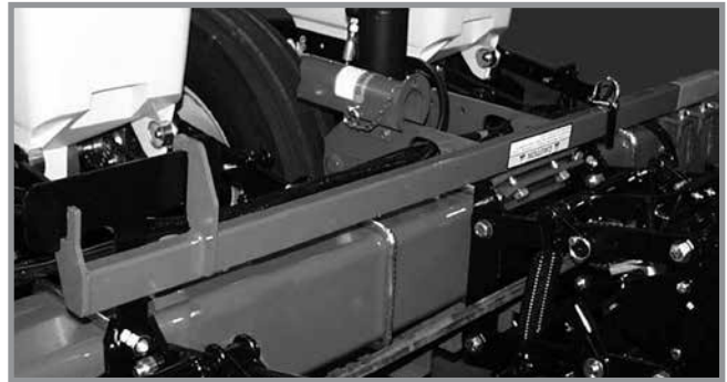
Lift lever in storage location
