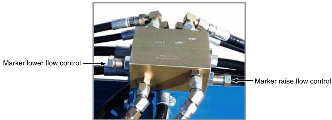
Row marker flow control valves
