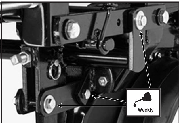
Row Unit Mounted Disc Furrower Parallel Linkages (6 Per Row)
