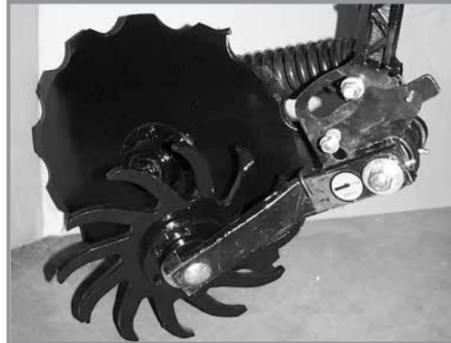
Notched single disc opener residue wheel attachment
