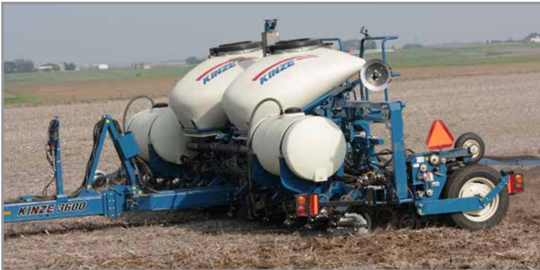
Liquid fertilizer installed on 3600 ASD
