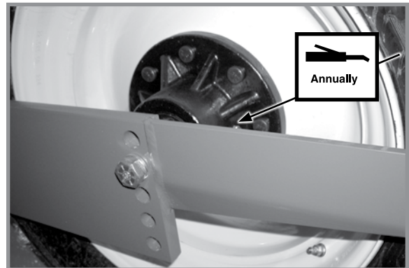
Transport wheel bearings - 1 per hub
