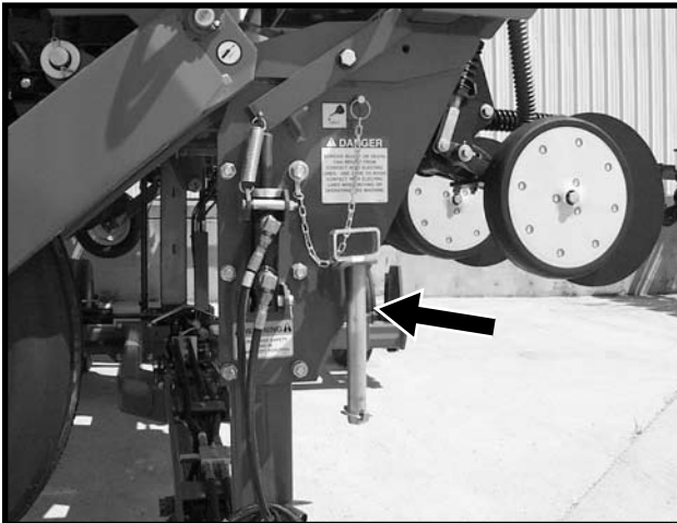
Tongue Safety Pin Stored For Field Operation
