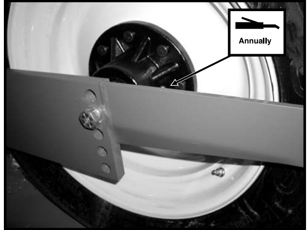
9. Transport Wheel Bearings - 1 Zerk Per Hub
