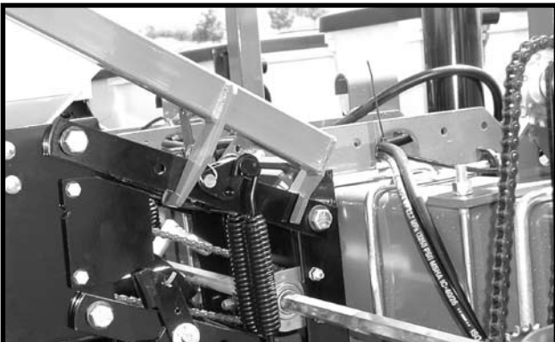
Lift Lever Positioned To Lift Push Row Unit
