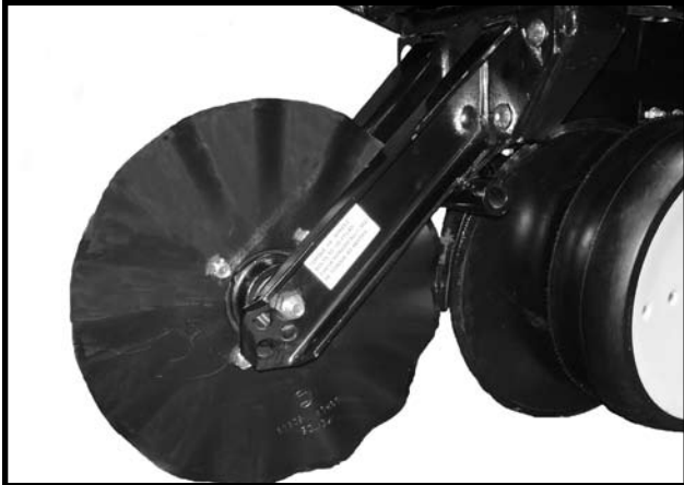
STYLE B (One Sleeve For Installing Coupler Mounted Residue Wheels)
