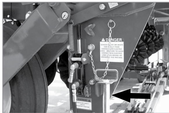
Tongue safety pin stored for field operation
