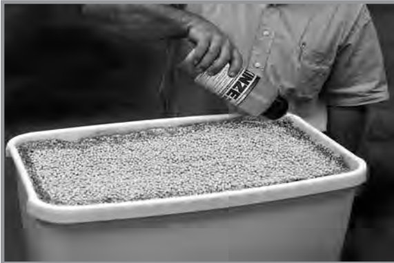
Adding graphite to conventional hopper
