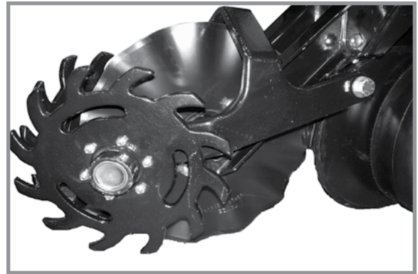
Coulter mounted residue wheels
