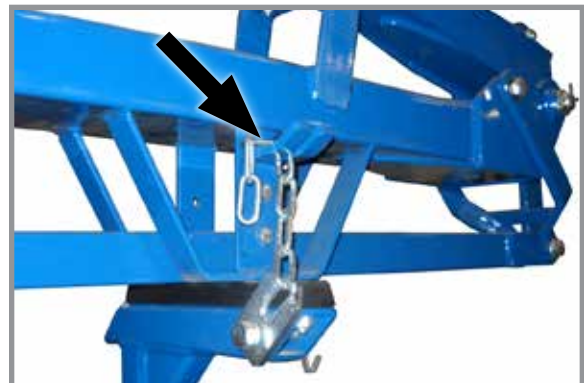
Row marker safety lockup installed
