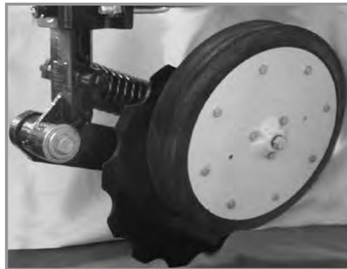
Notched single disc opener depth/gauge wheel
