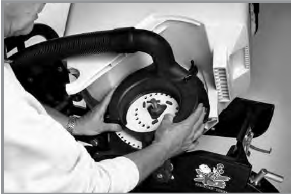
Remove vacuum cover and seed disc
