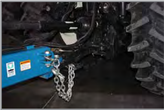
Planter/safety chain hookup to tractor
