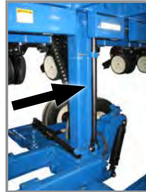
Safety lockup in transport/maintenance position
