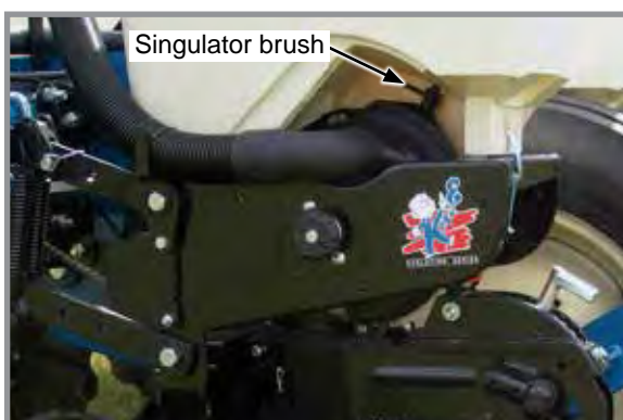
Singulator brush adjustment location
