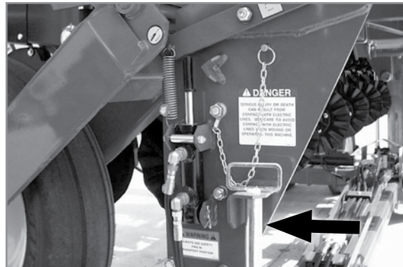
Tongue safety pin stored for field operation
