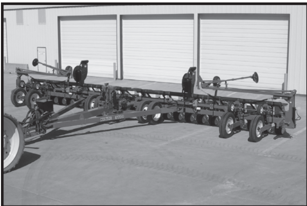
24 Row 22" Conventional Machine Shown In Field Operation Position
