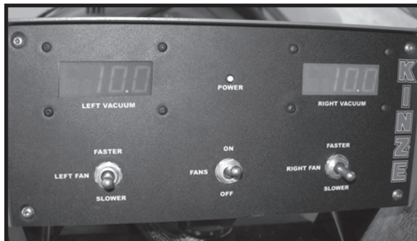
Vacuum Fans Control Console
