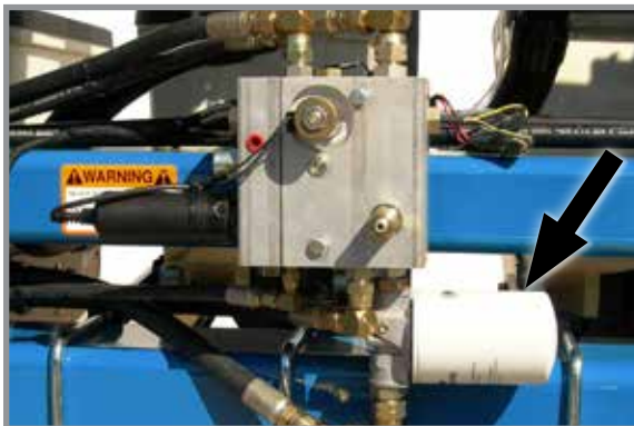
Oil filter location
