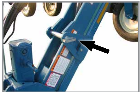
Hitch parallel linkage pin installed
