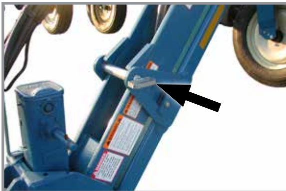
Hitch parallel linkage pin installed
