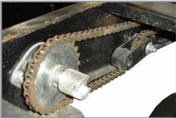
Row unit granular chemical drive
