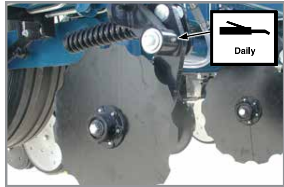
Notched single disc opener (1 per arm)
