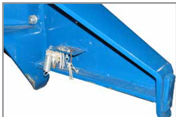
Spare shear pin storage
