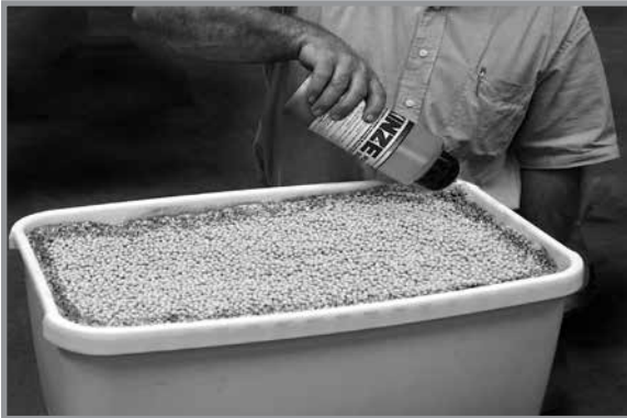
Adding graphite to conventional hopper
