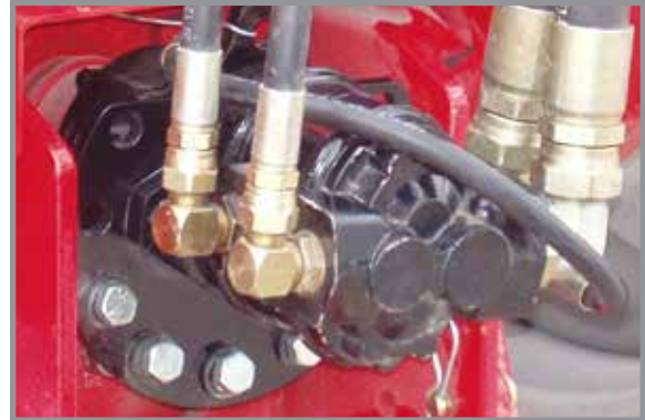
PTO pump installed
