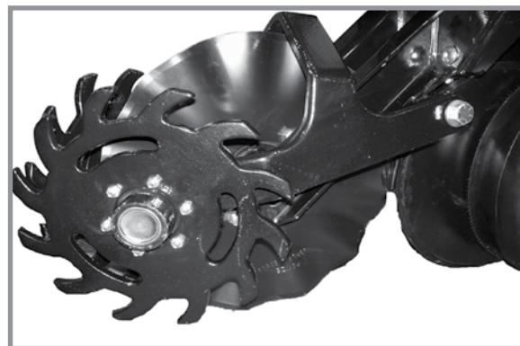
Coulters mounted residue wheels
