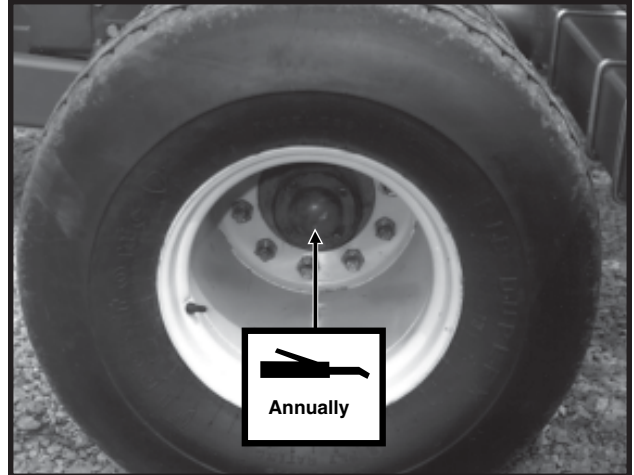
10. Transport Wheel Bearings - 1 Zerk Per Hub
