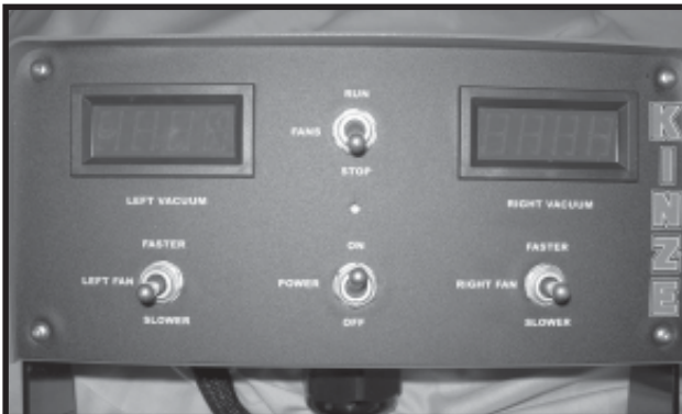
Digital Vacuum Gauges Control Console
