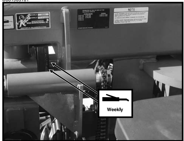
Inner End Of Stub Wing - 2 Zerks Per Assembly
