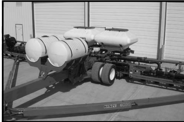
Model 3800 SDS EdgeVac® 36 Row 30" Planter With Liquid Fertilizer Package
