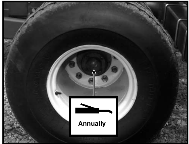
Transport Wheel Bearings - 1 Zerk Per Hub
