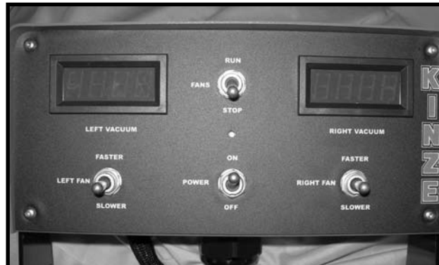
Digital Vacuum Gauges Control Console
