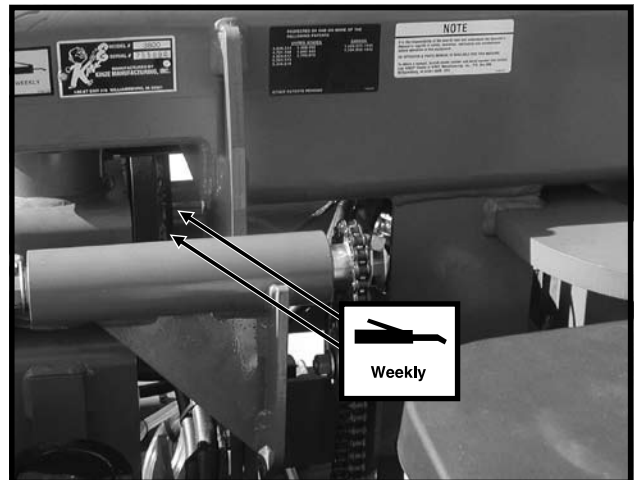
5. Inner End Of Stub Wing - 2 Zerks Per Assembly
