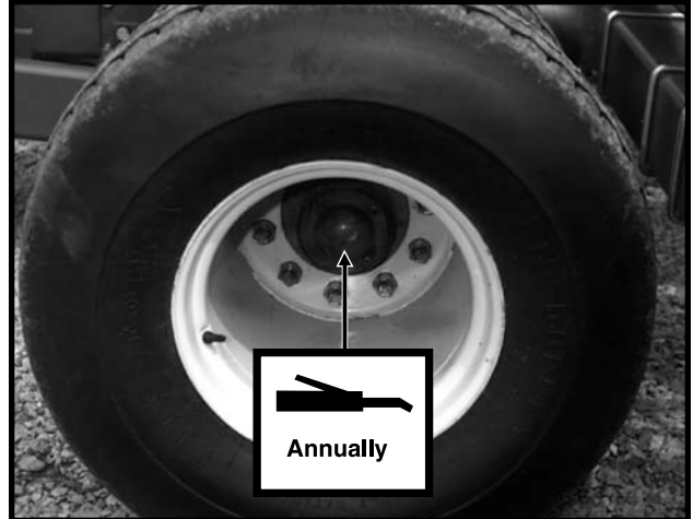
10. Transport Wheel Bearings - 1 Zerk Per Hub
