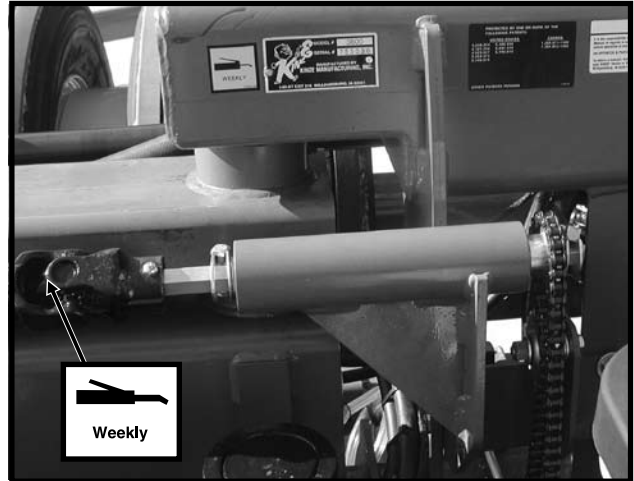
17. U-Joint Shaft Between Center Section And Wing - 1 Zerk On Each End Of U-Joint Shafts (2 Per U-Joint Shaft)
