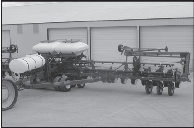
Model 3800 SDS 24 Row 30" With Optional Liquid Fertilizer Package, Notched Single Disc Fertilizer Openers And Piston Pump Package
