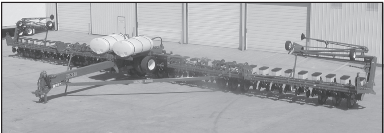
Model 3800 Conventional 36 Row 30" Planter With Optional Row Markers And Liquid Fertilizer Package
