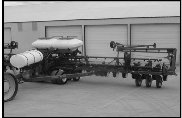
Model 3800 SDS 24 Row 30" With Optional Liquid Fertilizer Package, Notched Single Disc Fertilizer Openers And Piston Pump Package
