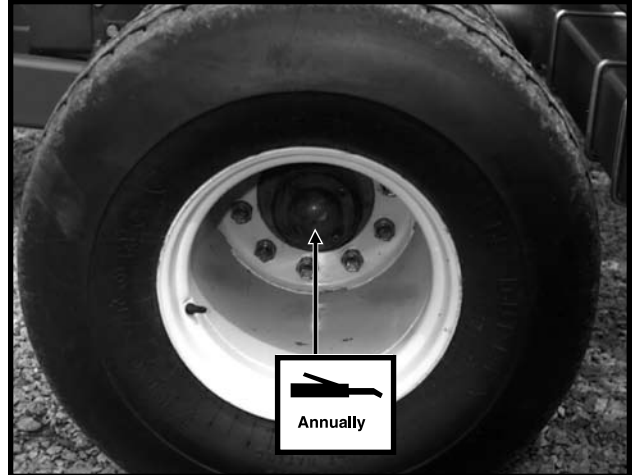
10. Transport Wheel Bearings - 1 Zerk Per Hub
