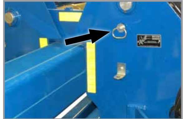
Wing latch hook safety pin installed
