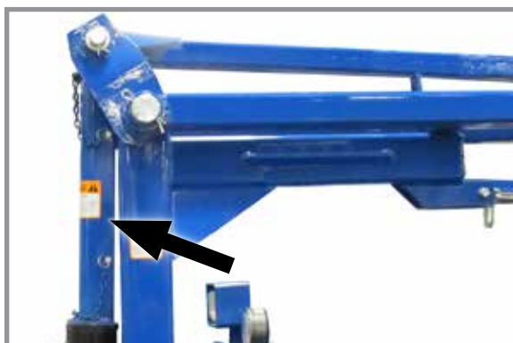
Marker arm safety lockup installed
