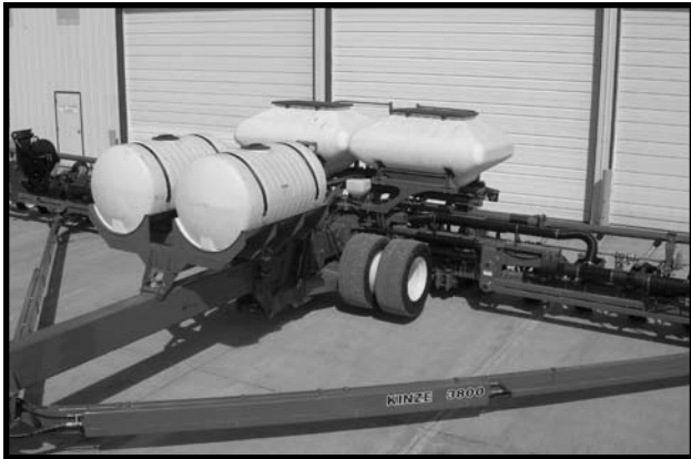
Model 3800 SDS 36 Row 30" With Optional Liquid Fertilizer Package, Notched Single Disc Fertilizer Openers And Piston Pump Package
