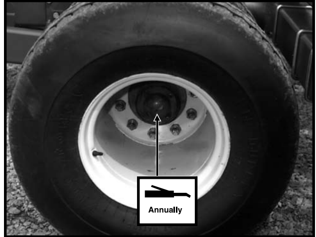
10. Transport Wheel Bearings - 1 Zerk Per Hub
