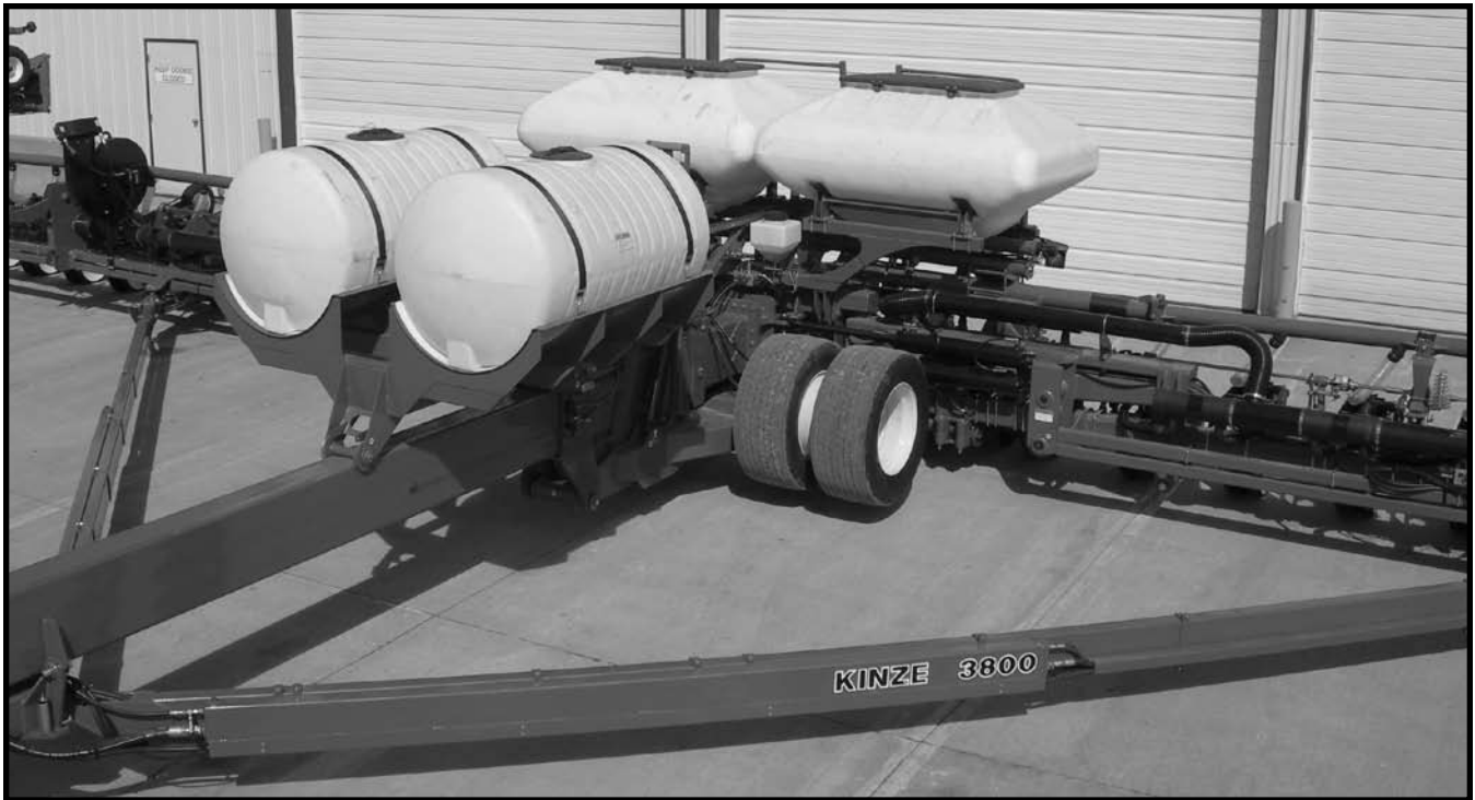
Model 3800 SDS 36 Row 30" With Optional Liquid Fertilizer Package, Notched Single Disc Fertilizer Openers And Piston Pump Package
