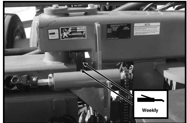
5. Inner End Of Stub Wing - 2 Zerks Per Assembly
