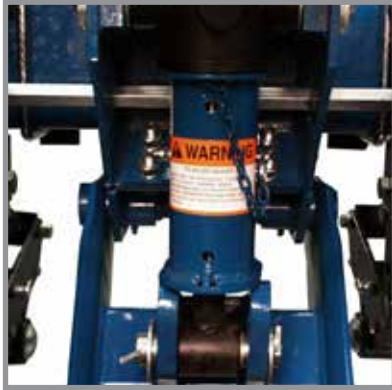
Safety lockup installed
