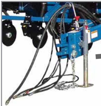
Jack stand installed
