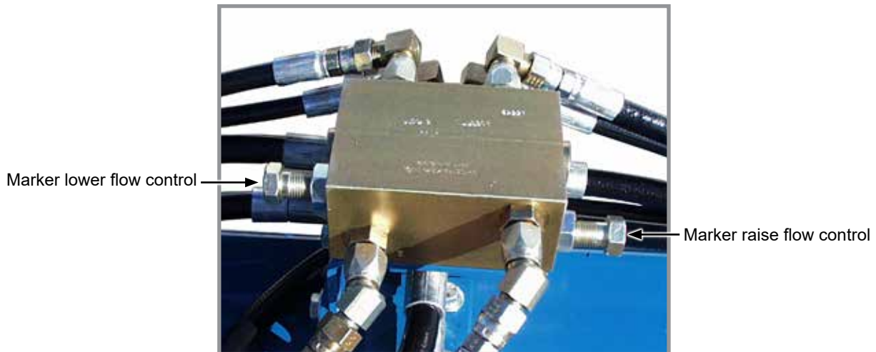
Row marker flow control valves
