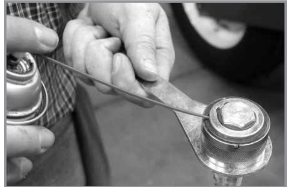
Wrap Spring Wrench Lubrication
