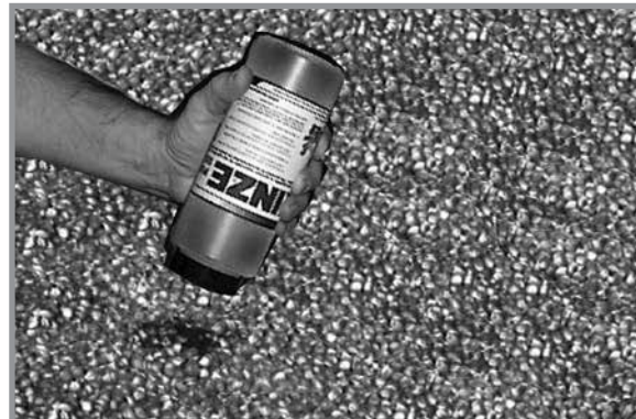
Adding graphite bulk fill hopper
