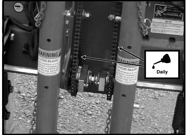
Center Drop Assembly Drive Chains
