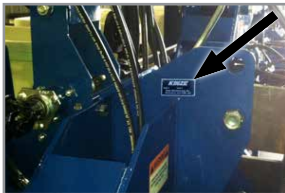
Serial number plate location - R.H. side of 3-point mount
