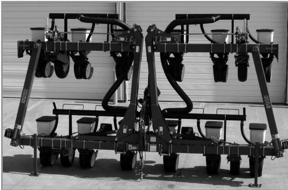
Model 3145 12 Row 38" Vacuum Planter (Less Optional Row Markers) Shown In Transport Position
