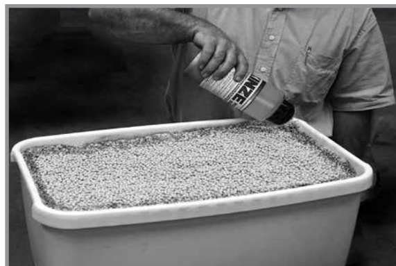
Adding graphite to conventional hopper
