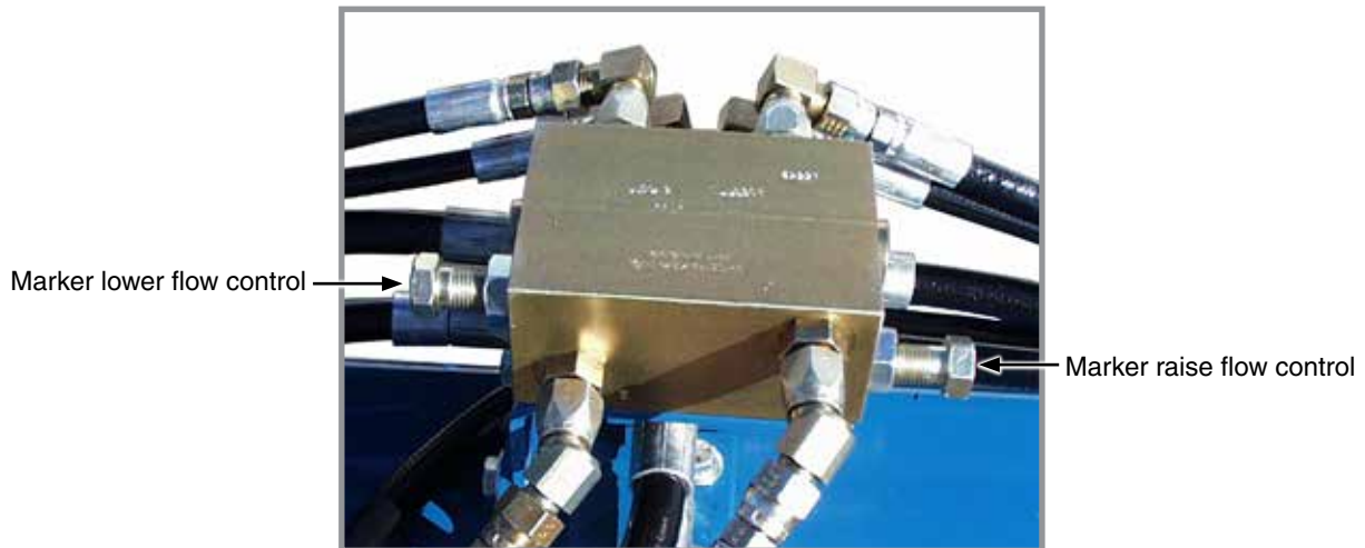
Row marker flow control valves
