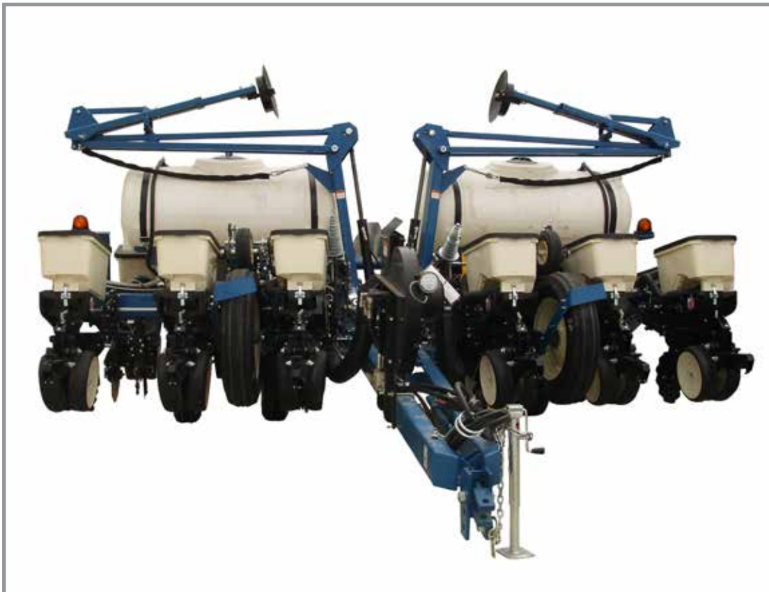
3200 Wing Fold Vacuum 12 row 30" with liquid fertilizer option (shown folded)
