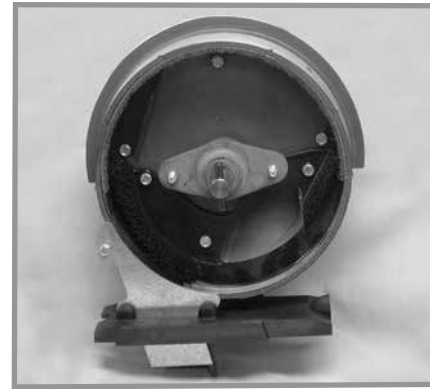
Shown without seed disc installed
