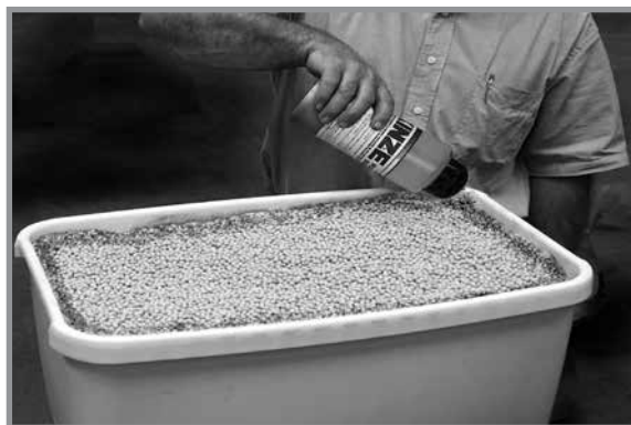
Adding graphite to conventional hopper
