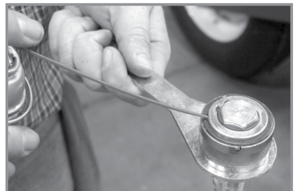
Wrap Spring Wrench Lubrication
