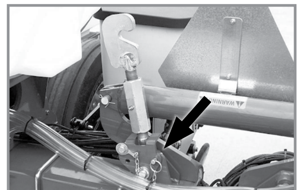
Center turnbuckle lockup pin
