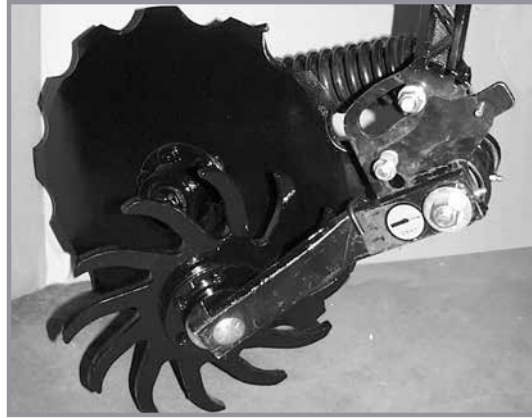
Notched single disc opener residue wheel attachment
