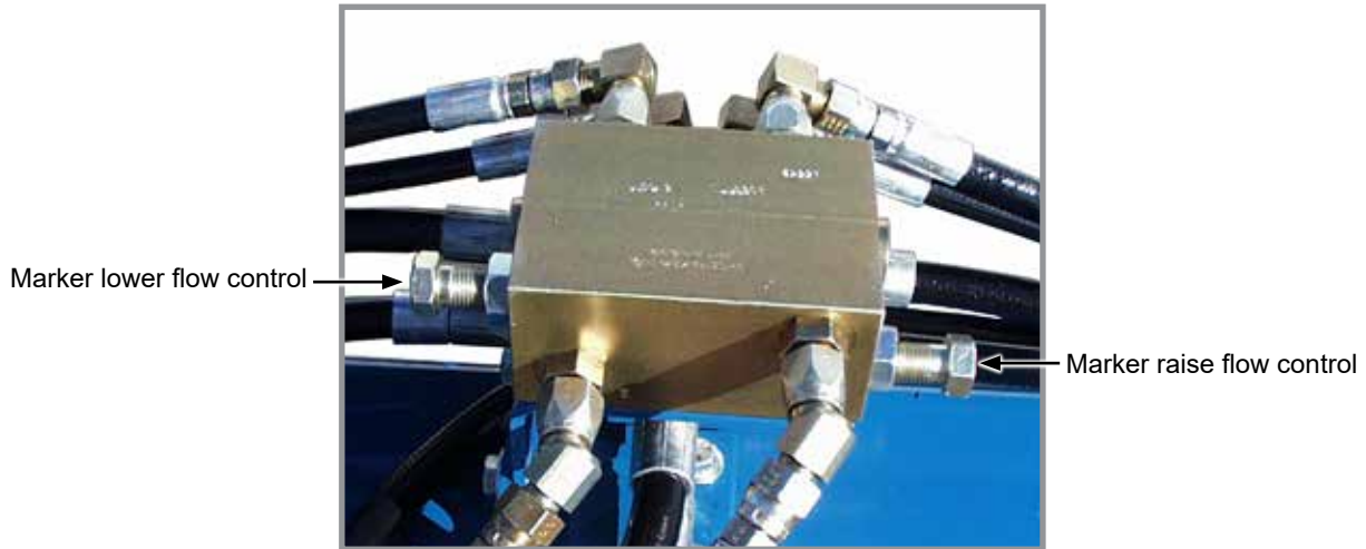
Row marker flow control valves
