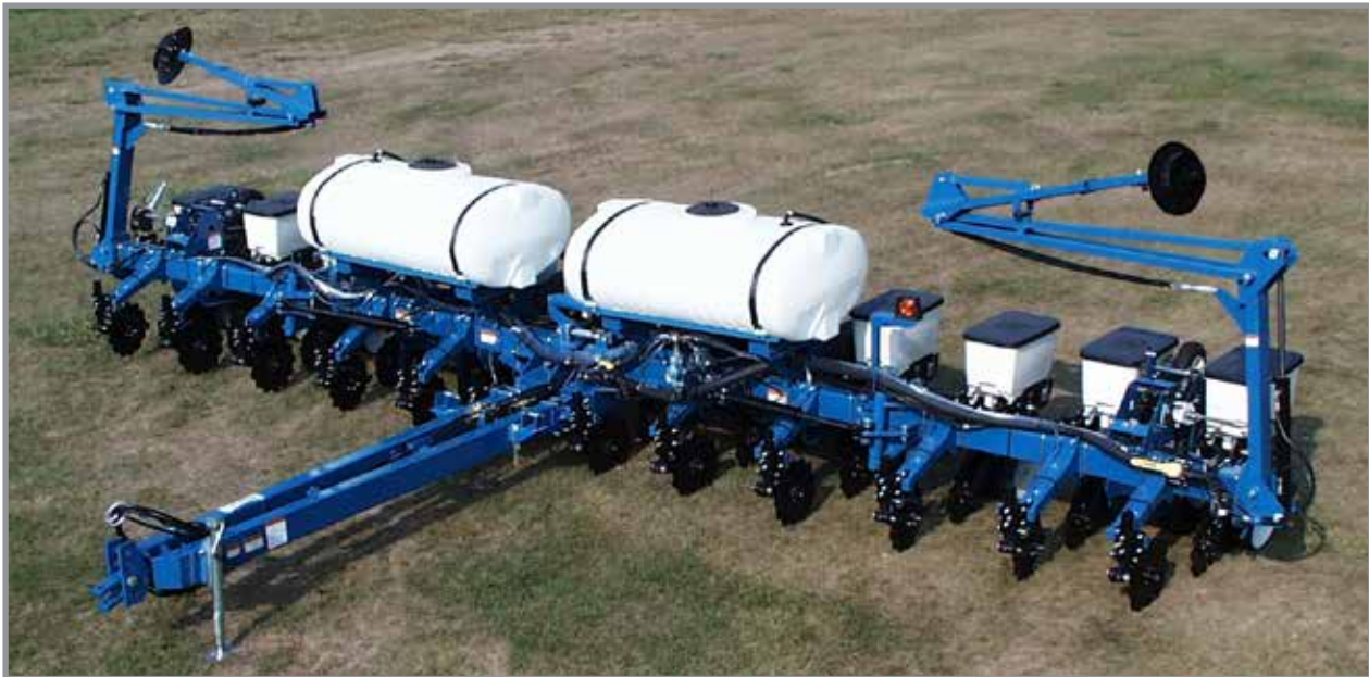
Liquid fertilizer option installed
