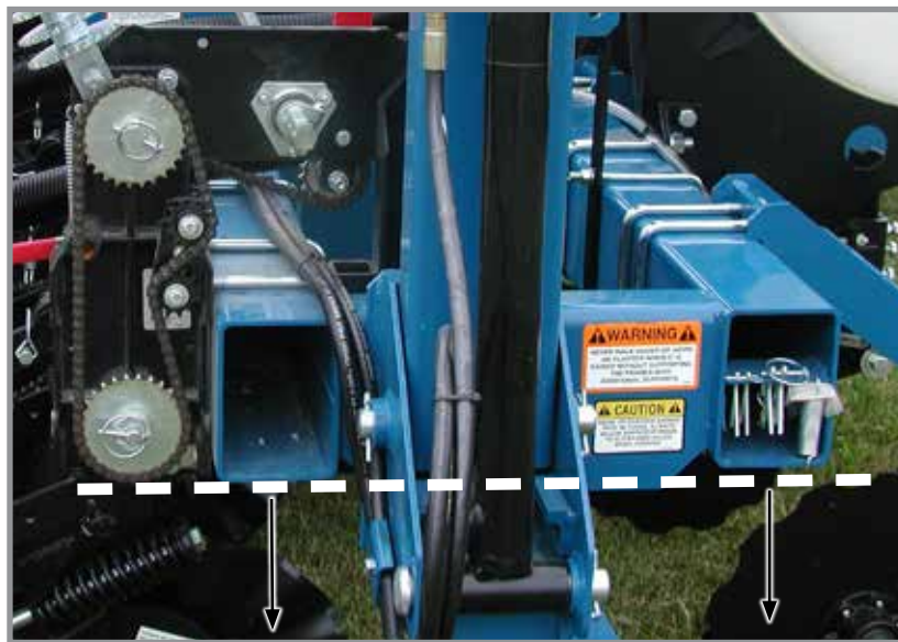
Bottom of toolbars 20" - 22" (50.8 - 55.8 cm) from planting surface
