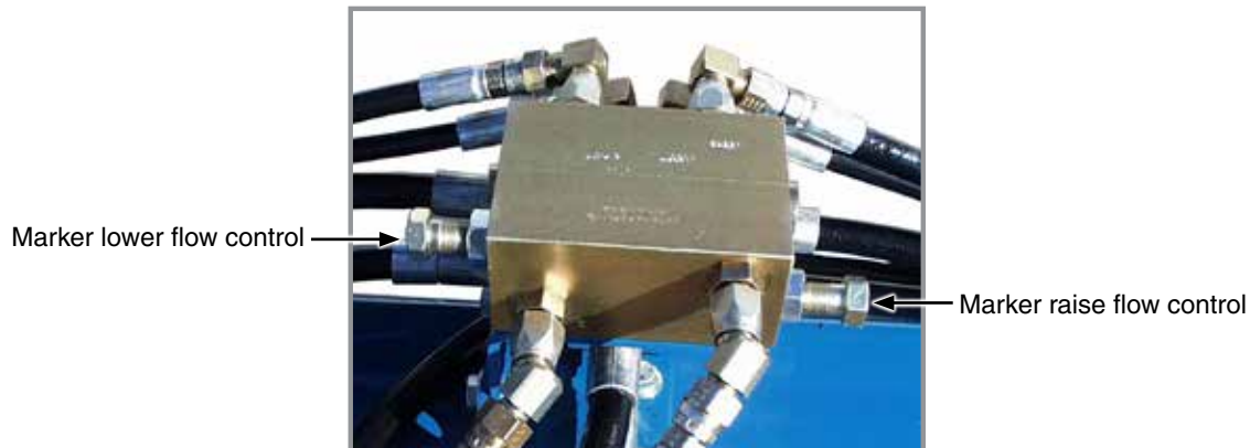
Row marker flow control valves
