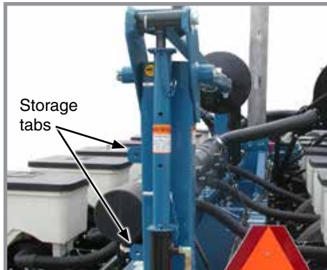
Row marker lockup installed
