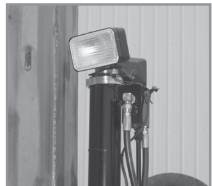
Auxiliary work lights
