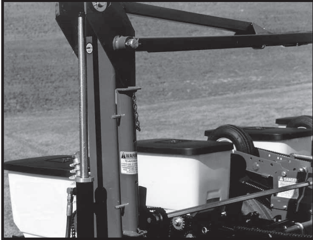
Lockup Stored For Marker Operation
